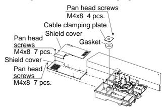
Figure 5-6 Antenna unit, inside view
